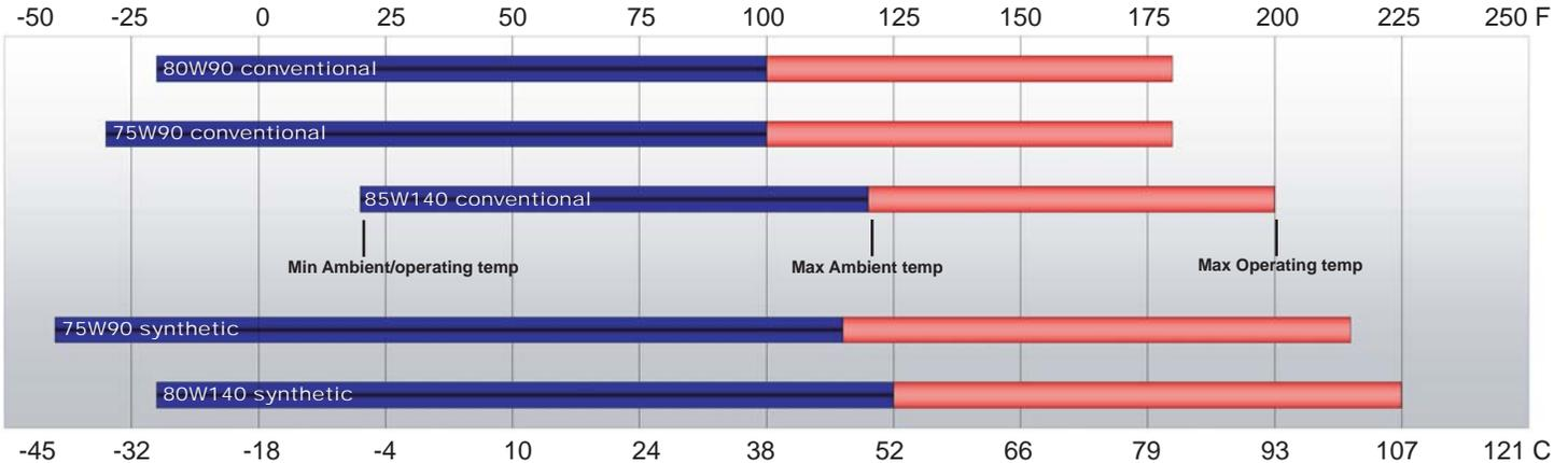
**Note:** Ambient temperature is the air temperature measured in the immediate vicinity of the gearbox. A Gearbox exposed to the direct rays of the sun or other radiant heat sources will operate at higher temperatures and therefore must be given special consideration. The max operating temp must not be exceeded under any circumstances, regardless of ambient temperature.
