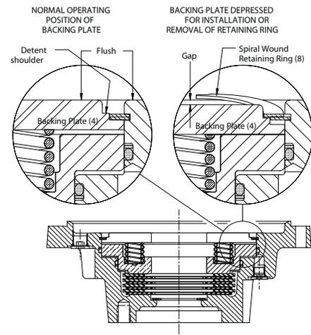
**NOTE:** The retaining ring (8) is normally under very high spring load. DO NOT attempt to remove it without first releasing spring load by depressing the backing plate (4) as described above. Personal injury and/or damage to the brake will result if this step is not followed.
