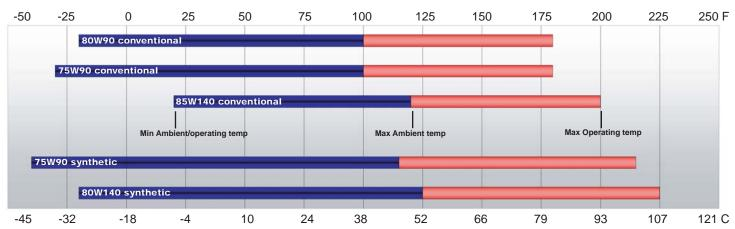
Note: Ambient temperature is the air temperature measured in the immediate vicintity of the gearbox. A Gearbox exposed to the direct rays of the sun or other radiant heat sources will operate at higher temperatures and therefore must be given special consideration. The max operating temp must not be exceeded under any circumstances, regardless of ambient temperature.
