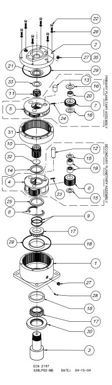
NOTE \* BEARING PRELOAD DETERMINES QUANTITY OF SHIMS.
