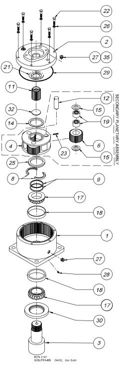
NOTE \* BEARING PRELOAD DETERMINES QUANTITY OF SHIMS.
