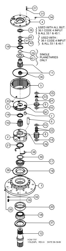
(\*) QUANTITY DETERMINED FROM BEARING PRELOAD.
