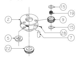
Rotate the planet gears (9) to check for abnormal noise or roughness in bearings (19) or planet shafts (7). If further inspection or replacement is required, proceed as follows:
